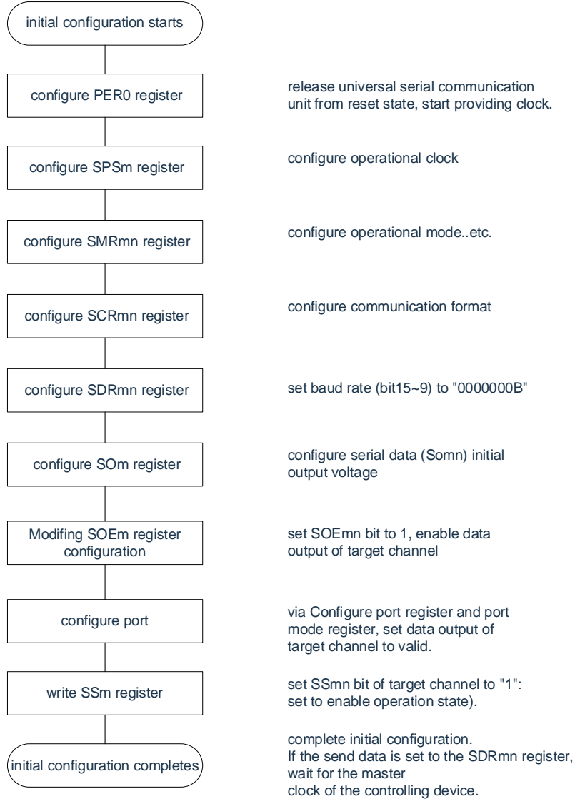
Figure 12-28: Initial setup steps for slave transmission
